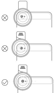
Screw the polarizer onto the clip.
